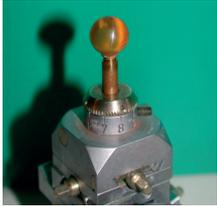
Fig.: Sphere of the nonlinear crystal  $\text{BaGa}_2\text{Se}_7$ , manufactured at NEEL Institute in Grenoble.
