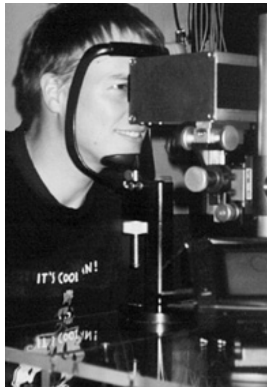
Figure 8 A test subject in front of the setup for blink reflex investigations
