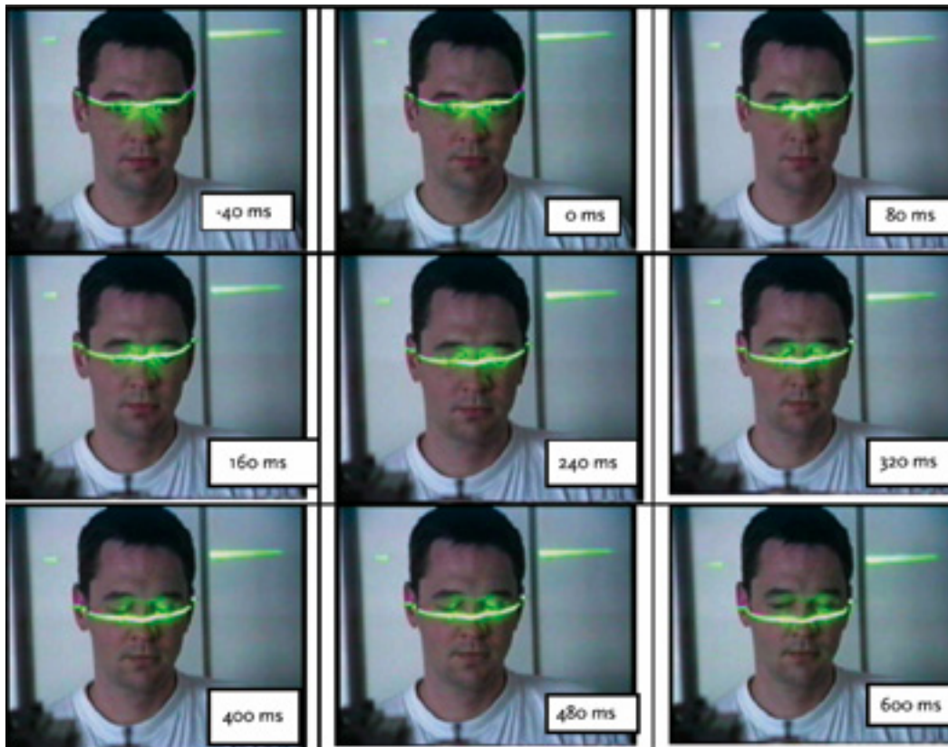
Figure 9 A laser line scanner test: vertical scanning motion of the laser line
